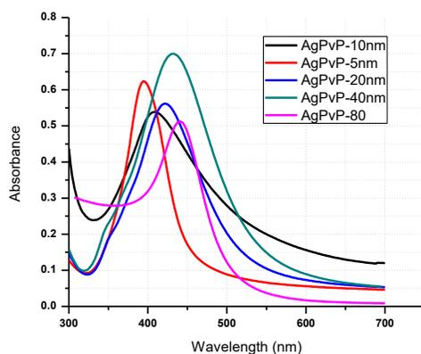
Fig. 2: Surface Plasmon Resonance Band of AgPVP nanoparticles of 5, 10, 20, 40, and 80 nm.
