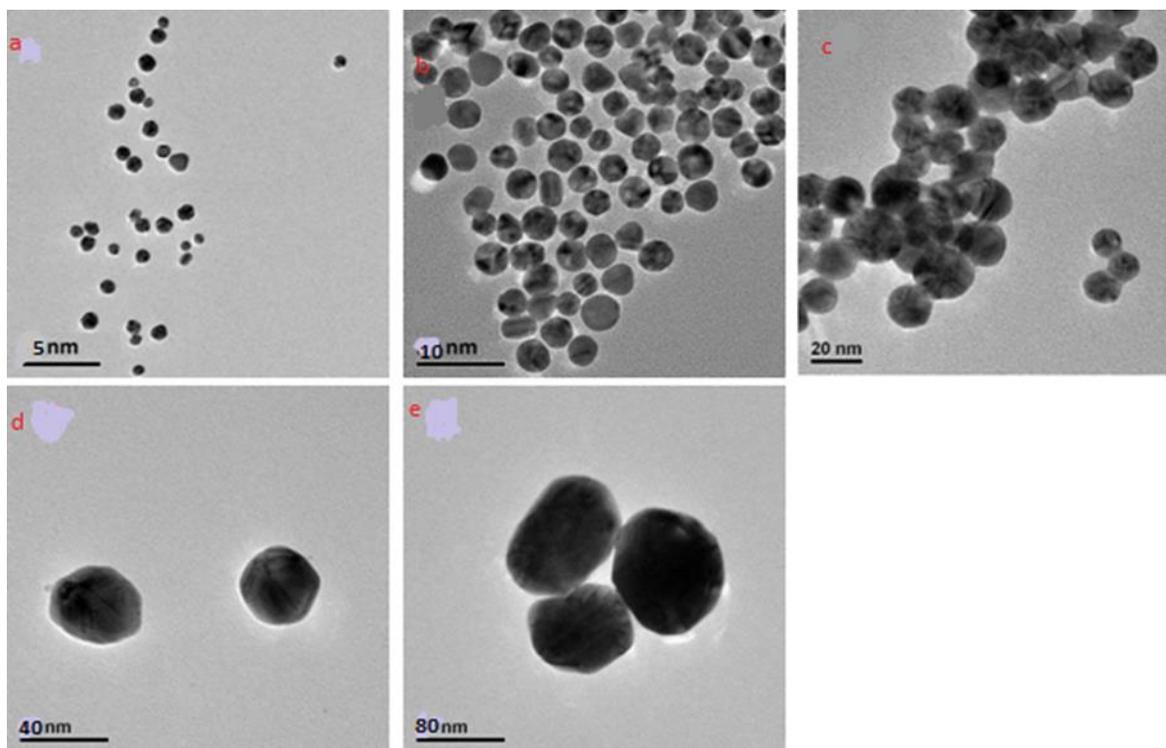
Fig. 3: TEM images of Silver nanoparticles capped with citrate (5nm(a), 10nm(b), 20nm(c), 40nm(d) and 80nm (e) in sizes).
